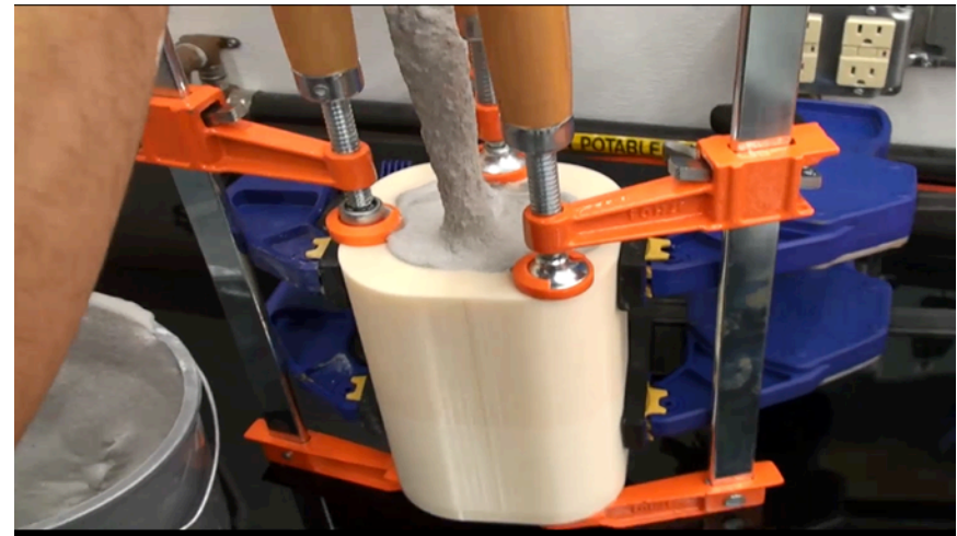
Forming sacrificial core in mold.
