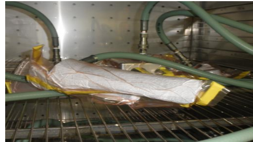
Thermal cure of vacuum-bagged composite part.
